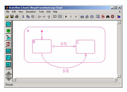
In this chart, transition 1 loops outside of logical parent A, which is the common parent of transition source B and destination C.
